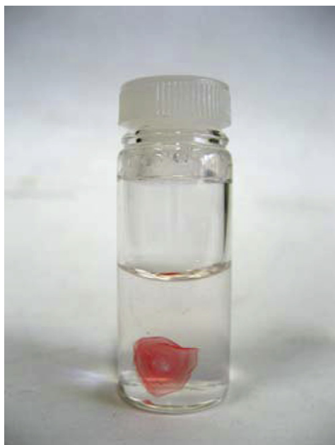
Fig. 2. Photograph of DNA–23 wt% SiNSi hybrid material in aqueous ethidium bromide solution. The hybrid material was dyed red by the accumulation of ethidium bromide.
